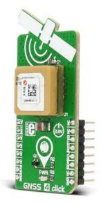
**GNSS 4 click** carries SAM-M8Q patch antenna module from u-blox. The click is designed to run on a 3.3V power supply. It communicates with the target microcontroller over I2C or UART interface.
