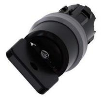
Key-operated switch O.M.R, 22 mm, round, plastic with metal front ring, lock number 73034, black, with 2 keys, 2 switch positions O-I, latching, actuating angle 90°, 10:30h/13:30h, key removal O, with laser labeling, inscription or symbol Customer-specific selection with SIRIUS ACT configurator (CIN)
