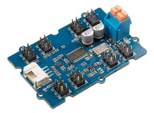
The Grove - 16-Channel PWM Driver is based on NXP PCA9685, which is a 16-Channel, 12 bit I2C PWM driver. This board can drive up to 16 servos with the external power supply. You can control this board with Arduino easily via the I2C Grove interface. In addition, you can use this board as a LED controller.
