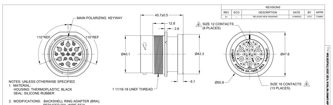
2. MODIFICATIONS: BACKSHELL RING ADAPTER (BRA); REDUCED DIA. WIRE SEAL.
