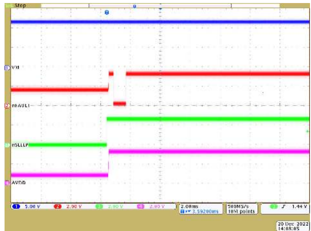
Figure 9-3. Device Power up with nSLEEP (VM, nFAULT, nSLEEP, AVDD)
