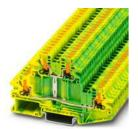
Protective conductor double-level terminal block, number of connections: 4, connection method: Push-in connection, 1st and 2nd level, Rated cross section: 4 mm², cross section: 0.2 mm² - 6 mm², mounting type: NS 35/7,5, NS 35/15, color: green/yellow
