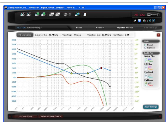
Figure 44 - Full loop gain and phase for Steady State load
