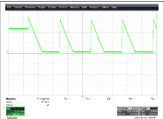
Figure 42 - Hysteretic VS3 Over Voltage Protection (set to 17V) Output voltage, 5V/div, 500ms/div
