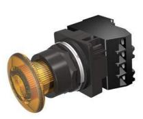
30mm BlackMax, Epoxy Coated Corrosion Resistant Complete Metal Unit Illuminated Push-Pull Operator Transformer type, 240V AC LED Lamp Mushroom Head Cap Small 1 3/4" (44.5 mm) Plastic, Amber 2 Position Maintained, Pull-to-Release with 1 N.O. - 1 N.C. Heavy Duty Contacts, A600/P600 UL Listed, CSA Certified NEMA 1,3,3R,4,4X,12,13 & Automotive Standards
