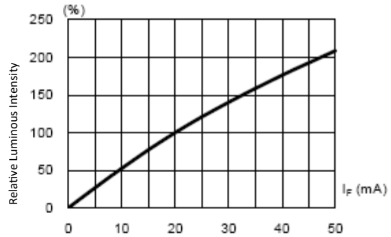
Fig. 2 Luminous Intensity vs. Forward Current
