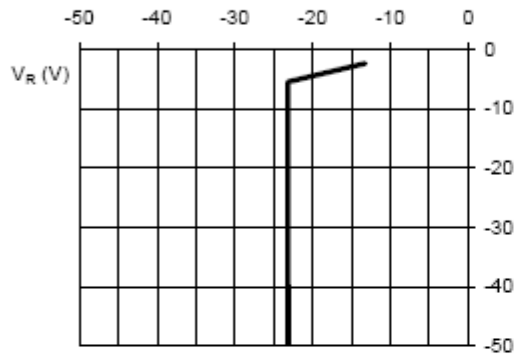
Fig. 3 Reverse Current vs. Reverse Voltage I_R ( \mu A)
