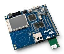
\* Photo of the SPB104 in one of the SD-card slots on the EVK1104. Ready-made downloadable reference designs can up and running within minutes and development can start at once. The SPB104 is fully tested and calibrated and is targeted for a good "out-of-the-box" experience together with the AVR32 platforms such as the EVK1004, see <a href="https://www.atmel.com/wifi">www.atmel.com/wifi</a>
