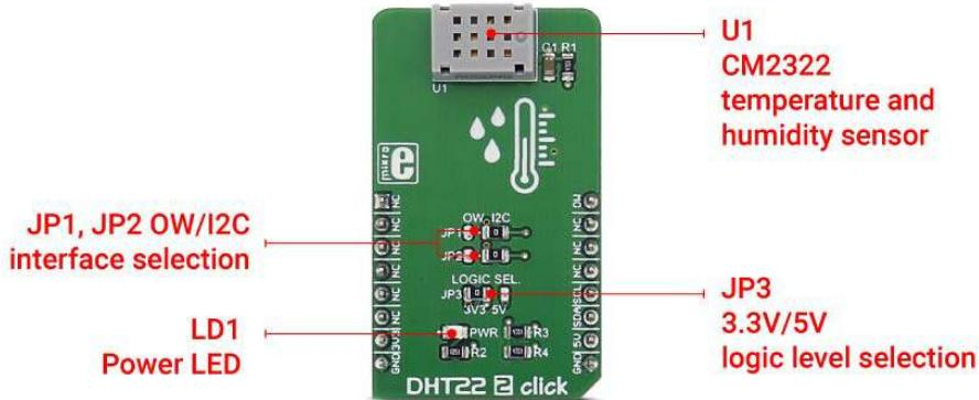
Typical temperature accuracy is  $\pm 0.3^{\circ}\text{C}$ , while relative humidity accuracy is 2% RH, with the resolution of 0.1 for both measured properties.
