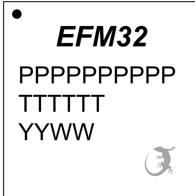
Figure 10.3. QFN64 Package Marking
