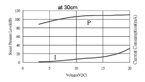
P: Voltage vs. Sound Pressure Level I: Voltage vs. Current Consumption
