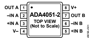
Figure 3. 8-Lead MSOP (RM-8)
