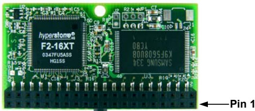
Figure 4: iDiskOnChip Horizontal Version 40 pin, Right-Oriented
