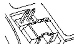
Figure 9: Master Setting for Vertical iDiskOnChip 40-Pin Connector
