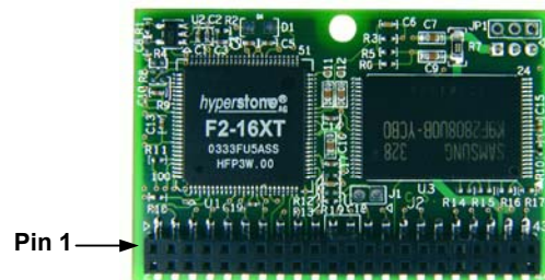
Figure 5: iDiskOnChip Horizontal Version 44 pin, Left-Oriented
