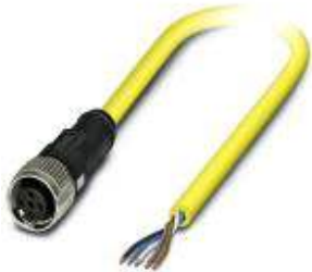
Sensor/Actuator cable, 5-position, TPE, yellow RAL 1021, free cable end, on Socket straight M12 SPEEDCON, A-coded, Cable length: 10 m
