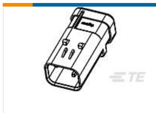
TE Part #776536-3 AS 16, 4P CAP ASSY, RD, KEY 3
