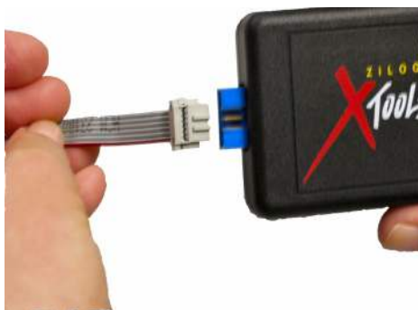
Figure 2. Connecting the Six-Conductor Ribbon Cable to the USB Smart Cable
