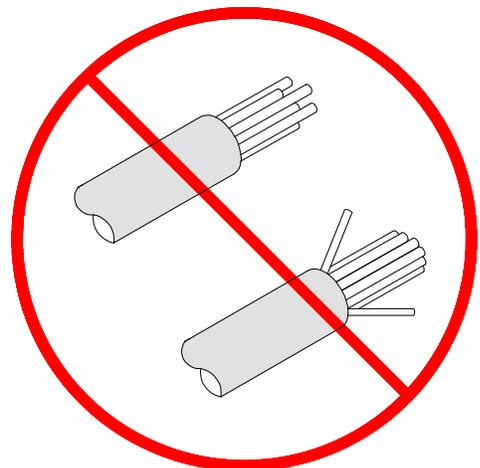
**Note:** Due to the delicate nature of this wire, care must be taken to gently touch the wire to the wire stop when crimping. The wire must be positioned directly above the terminal. Pushing the wire against the wire stop will result in strands out of the crimp. For semi-automatic crimping the operator may choose to lay the wire into the terminal for crimping.
