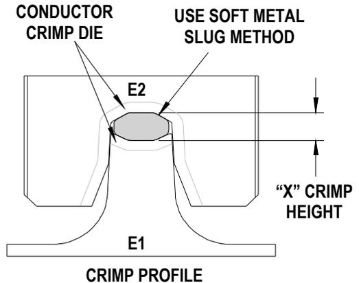
Use soft metal slug (solder) method to Measure the "X" dimension. Verify tooling crimp height calibration by referring to the Go/No Go dimensions shown in the chart.
