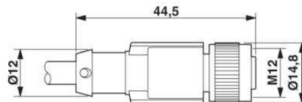
Socket M12 x 1, straight, with LED
