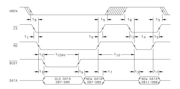
FIGURE 5. Slow memory mode, two byte read timing diagrams.
