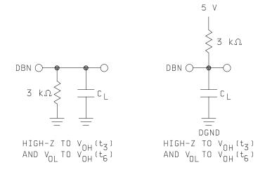
FIGURE 2. Load circuit for access time.
