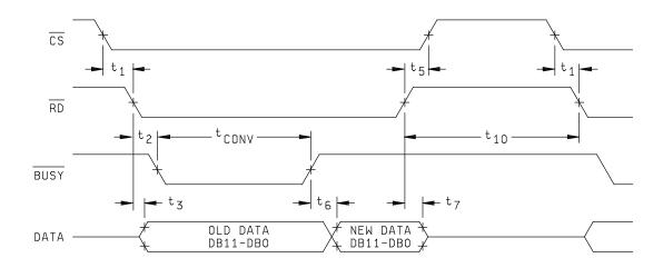
FIGURE 4. Slow memory mode, parallel read timing diagrams.
