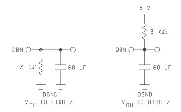
FIGURE 3. Load circuit for bus relinquish time.
