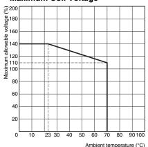
Note. The maximum allowable voltage is the maximum possible value of the voltage that can be applied to the relay coil.
