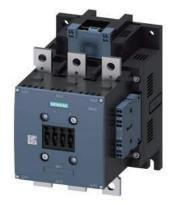
power contactor, AC-3e/AC-3 300 A, 160 kW / 400 V, Uc: 24 V DC x (0.7-1.25) PLC input 24-110 V DC 3-pole, auxiliary contacts 2 NO + 2 NC drive: electronic main circuit: busbar control and auxiliary circuit: spring-loaded terminal extended rated condition railroad IEC 60077
