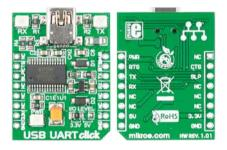
USB UART Click<sup>™</sup> is an accessory board in **mikroBUS<sup>™</sup>** form factor. It's a compact and easy solution for adding serial UART communication via USB cable. It features **FT232RL** USB-to-UART interface module as well as USB MINI B connector. USB UART Click<sup>™</sup> communicates with target board via UART interface. The board is designed to use 3.3V or 5V I/O level. It has a LED diode (GREEN) that indicates the presence of power supply.
