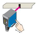
When setting the contrasts to be detected, "1st" flashes. Press set button.
