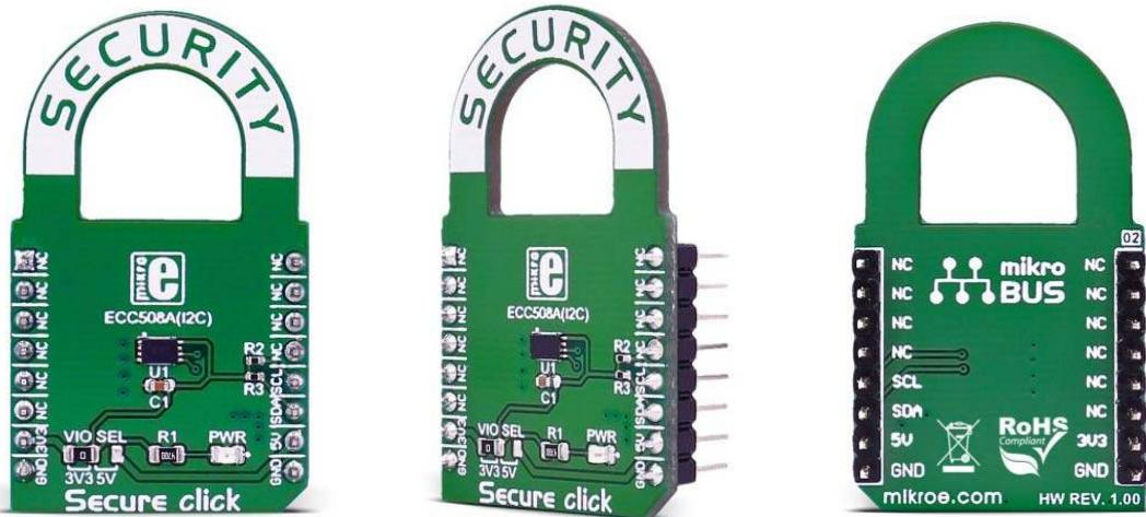
**Secure click** carries the ATECC508A cryptographic coprocessor with secure hardware-based key storage. The click is designed to run on either 3.3V or 5V power supply. It communicates with the target microcontroller over I2C interface.
