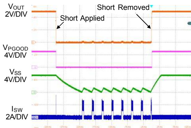
Figure 3. Short Circuit Protection and Recovery
