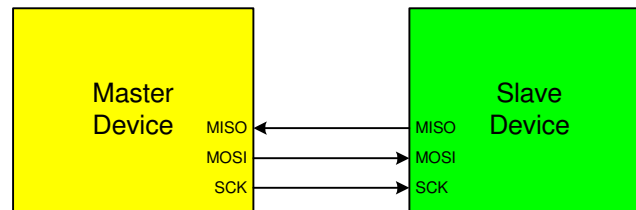
Figure 16.3. 3-Wire Single Master and Slave Mode Connection Diagram
