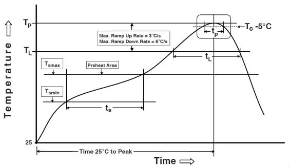
Preheating temperature:  $150 \sim 180$ °C,  $90\pm30$  seconds Liquidus temperature (TL): 230°C,  $30\pm10$  seconds
