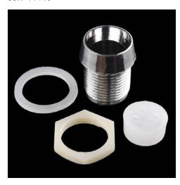
**Description:** These plastic LED holders have a slick chrome finish and make it possible to panel-mount your indicator lights for a clean look. These LED holders accept a 10mm LED and mount into an ½" diameter hole.
