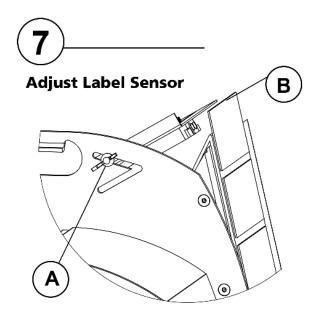
A: Loosen wing screw, then adjust sensor plate.B: Point sensor towards the top edge of the label.C: Tighten wing screw to secure sensor in place.
