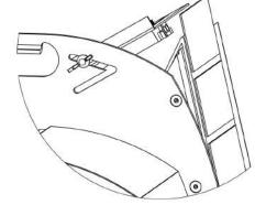
A: Feed label liner over strip plate separating the liner from the label
