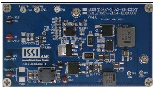
Figure 1 Photo of IS32LT3957/IS31LT3957 Boost Evaluation Board
