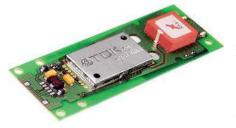
Most electronic equipment that gathers data has a serial port for offloading that data. This generally requires a hard wire connection by means of a serial cable. The TDK BISM is a module that can be incorporated into an existing design to provide a wireless serial connection between two devices. This allows for the remote
