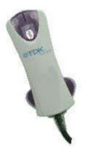
This device connects to the USB port of a laptop or desktop and can be used as a transmitter/receiver to communicate with other Bluetooth devices (e.g. partner with BISM module). This product does not have the built in software stack and requires additional drivers. The drivers are included on a CD that comes with the adaptor. This product can also be used to communicate with any other Bluetooth device, industrial or commercial.
