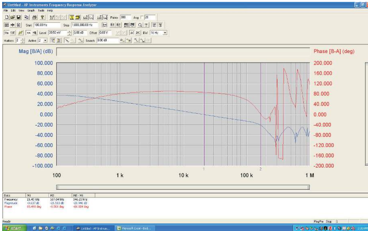
Figure 8-10. Bode Plot at 12 V IN , 1.1 V/25 A
