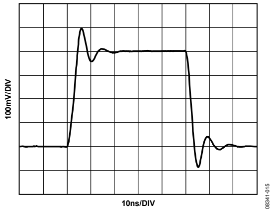
Figure 40. Small Signal Transient Response, G = 12.04 \text{ dB}
