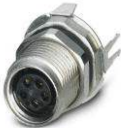
Sensor/actuator flush-type plug-in connector, socket, 5-pos., DeviceNet, M8, rear/screw mounting with M10 fastening thread, with straight solder connection
