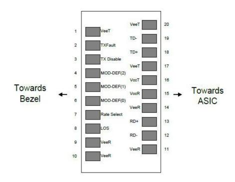
Pin-out of connector Block on Host board
