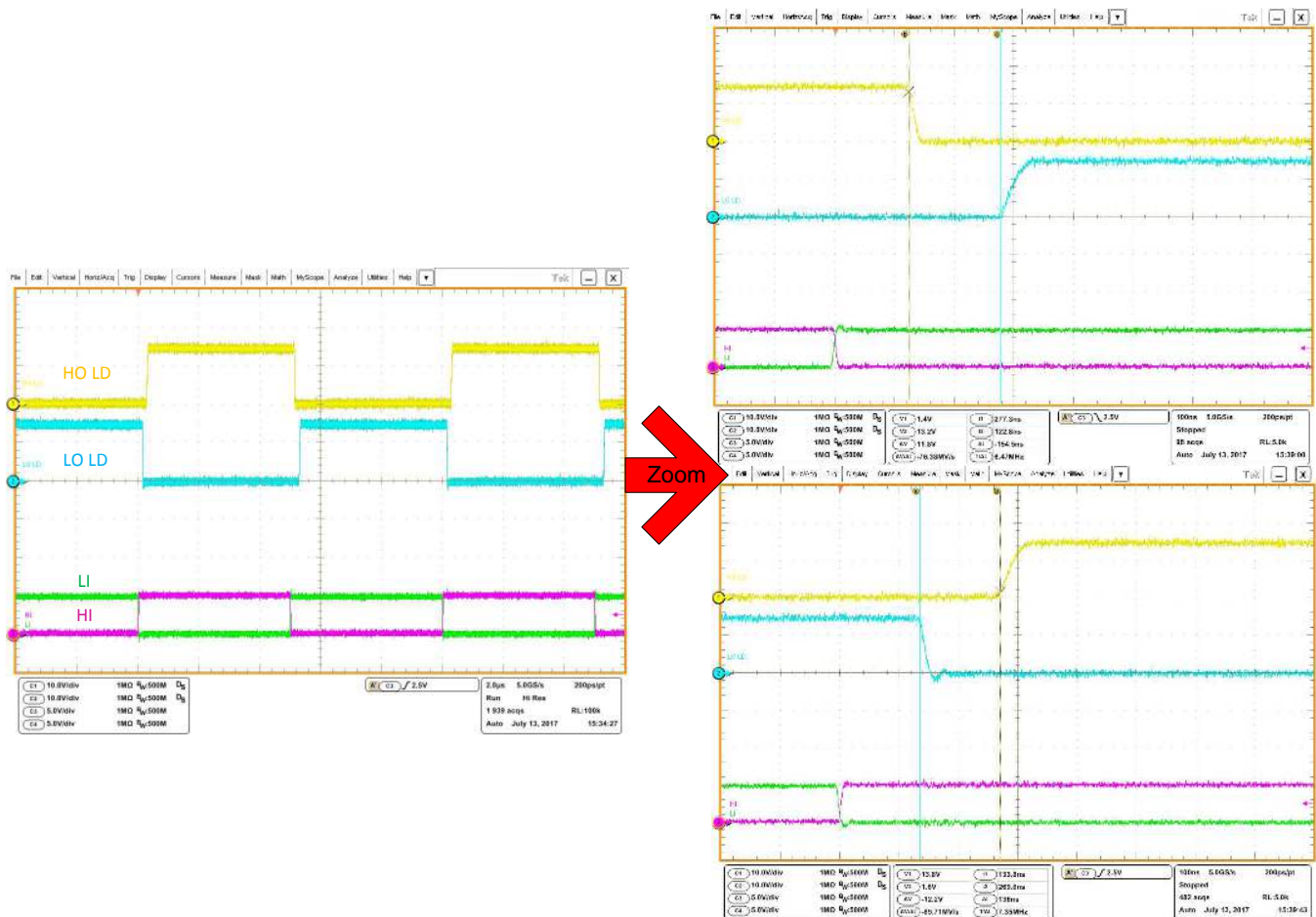
Figure 2. Example Input and Output Waveforms with Complimentary Input Signals (Green and Magenta are PWM Inputs, Yellow and Blue are Driver Outputs)
