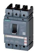
molded case switch 3VA5 UL frame 250 max. sh-circ breaking capacity 100kA @ 480V 3-pole, line protection MCS110, In=100A without overload protection self-protection li=16 x In without connection
