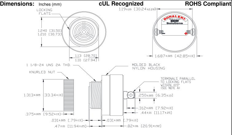
PLATED, TAPPED FOR #6-32 SCREW. TWO #6-32 NICKEL PLATED BRASS SCREWS INCLUDED. WILL ACCEPT 1/4" QUICK CONNECT.
