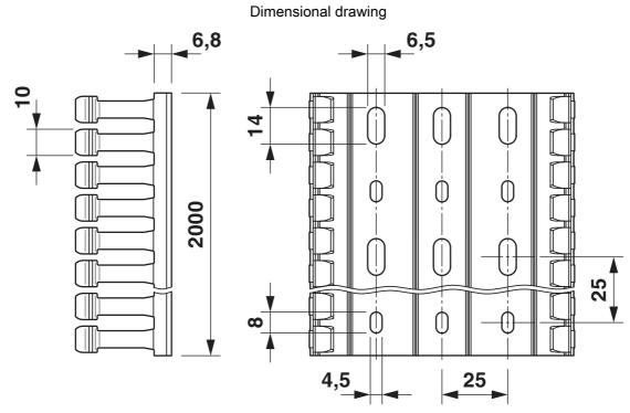
Base perforation according to DIN EN 50085
