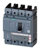
circuit breaker 3VA5 UL frame 250 breaking capacity class C 100kA @ 480V 4-pole, line protection TM210, FTFM, In=250A overload protection Ir=250A fixed short-circuit protection Ii=10 x In N conductor protection 100% without connection
