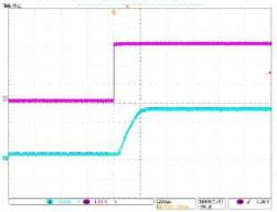
Load Transient Io=0~2A, Vo=3.3V, Vin=5V
