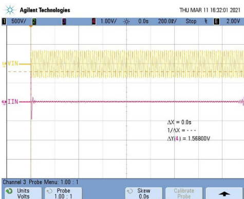
Inrush Current; 264Vac Input, Cold Start, Full Load; 31.4Apk
