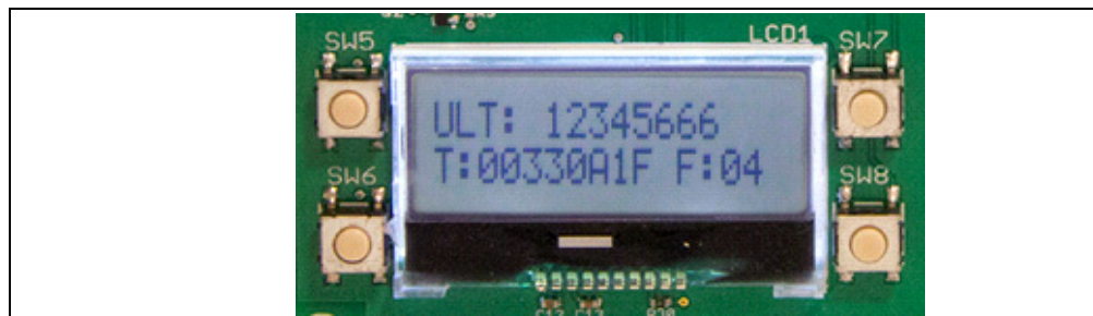
FIGURE 2-6: TYPICAL ULTIMATE KEELOQ ® TRANSMISSION
