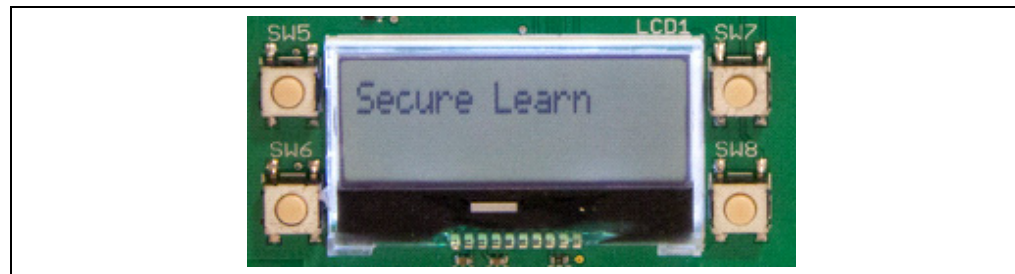
FIGURE 2-8: ENTER SECURE LEARN MODE
