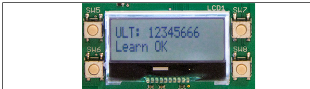
FIGURE 2-12: ULTIMATE KEELoQ ® PAIRING COMPLETE
