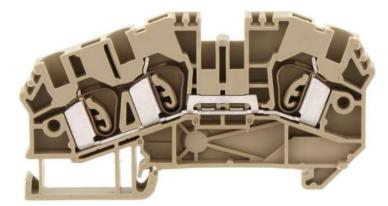
Ex feed-through terminal ATEX-certified, Tension-spring connection, Mounting type: Mounting rail TS 35/7.5, Rated cross-section: 4 mm<sup>2</sup>, Width: 6.1 mm, Colour: Beige
