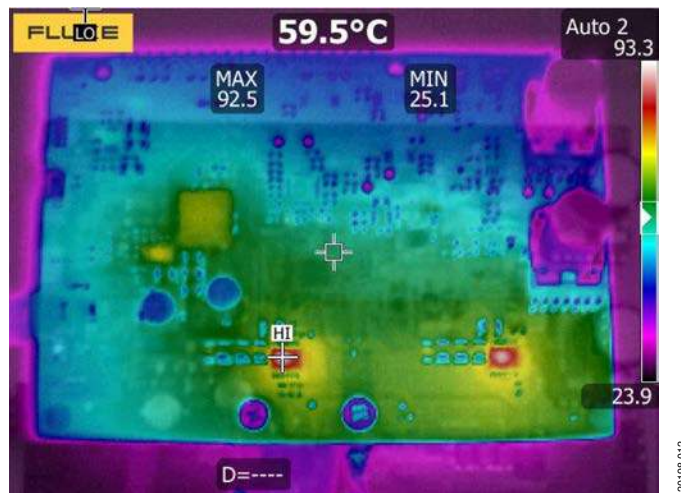
Figure 11. Thermal Image of EVAL-CN0508-RPIZ at 30 V Input, 2.75 A Current-Limit Output into 4 Ω Load
