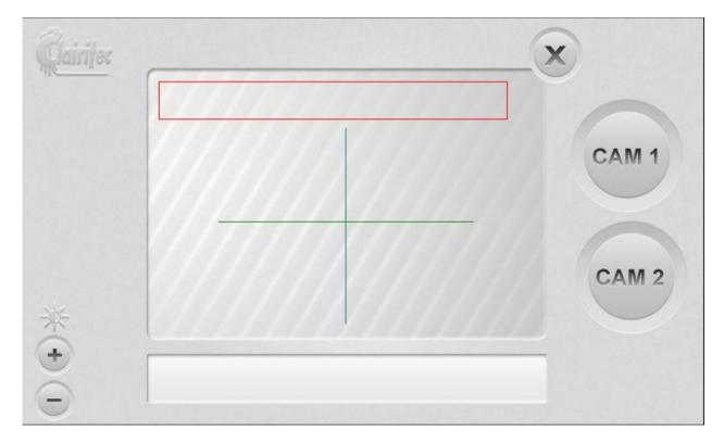
The HMI screen is composed out of 6 touchable buttons, 2 text zones, a red rectangle, and two lines (green and blue). All of these elements have been placed with the HMI Editor of GraphConverter.
