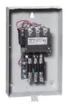
Non-reversing motor starter, Size 2 1/2, Single phase, 2-pole, Amb compensate bimetal OLrelay Contactor amp rating 60Amp 110 120/220 240VAC 60HZ coil, Non-combination type, Enclosure type 1, Indoor general purpose use
